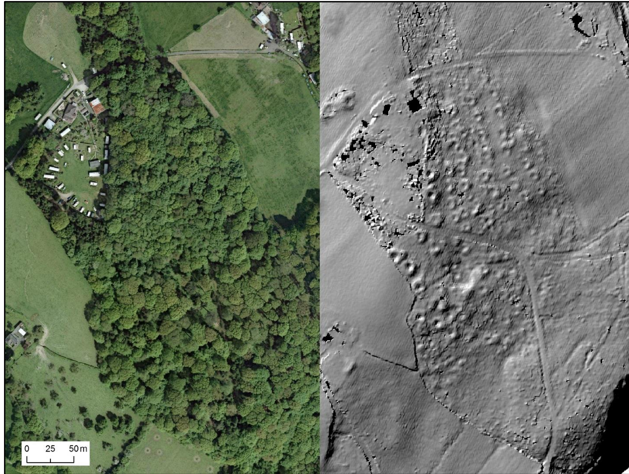
Figure 25. Cliff Wood, Hawkbatch, north of Bewdley, Worcestershire. The woodland in the photograph appears on the provisional ancient woodland inventory as ASNW. The processed LiDAR hillshade image on the right allows us to ‘see into the trees’ and find a cratered landscape. The craters are the traces of historic coal mining, spoil having been arranged around the openings of a series of shafts. The site was worked for a relatively short period in the early part of the 17th century with the coal being transported away on the River Severn, which is just to the east of the wood (information courtesy of Adam Mindykowski, Worcestershire Archive & Archaeology Service). Aerial photograph © 2015 Getmapping plc and Bluesky International Ltd. LiDAR images © Worcestershire Archive and Archaeology Service. Based on data supplied by the Unit for Landscape Modelling and Forest Research as part of the Grow with Wyre Project. No further copies may be made.
